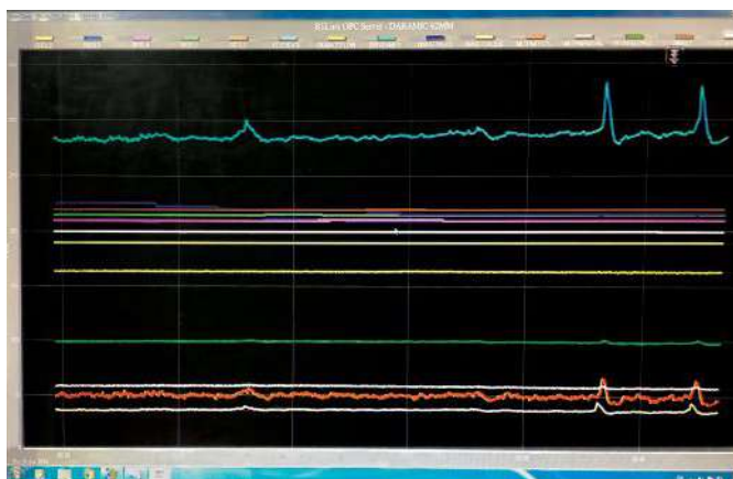
FIG 4 Upset conditions are extremely hard to diagnose since the parameter always returns to the initial equilibrium condition after the upset. There is no pattern or regularity for the time between upset conditions or the amount of deviation during the upset condition.
