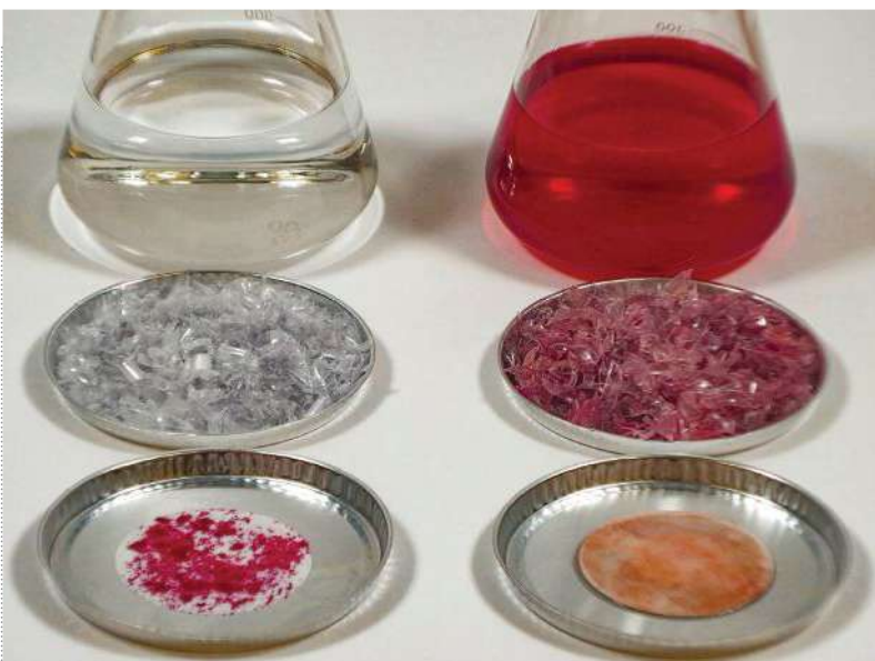
After being isolated from the bath, the SolvaWash product on the left comes out clean and clear, compared with traditional ink on the right.
