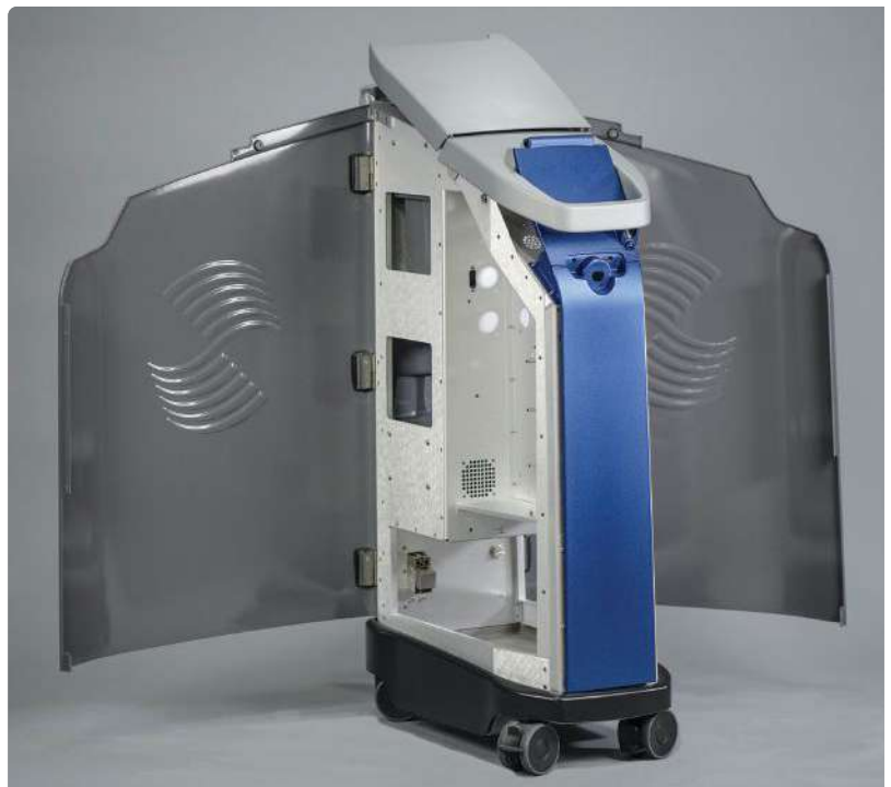
The 12 pressure-formed parts of this medical cart have no outside attachments, and undercut features are used to secure the side panels. When the side panels are closed, other parts in the assembly overlap to hide any additional attachment hardware. (All photos: Ray Products)
