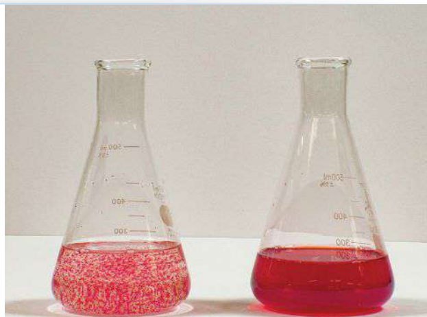
Sun Chemical's SolvaWash ink product on the left compared with conventional ink on the right. SolvaWash washable ink releases from the film in a controlled process that generates particles large enough to be easily filtered and removed from the wash solution. (Photos: Sun Chemical)
