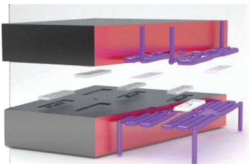
Generic example of a multicavity mold for COVID test kits, with conformal cooling.
