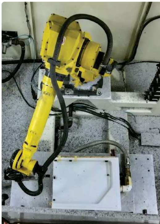
Ray develops tight-tolerance, highly aesthetic enclosures and utilizes equipment like this six-axis robotic CNC trimming center.
