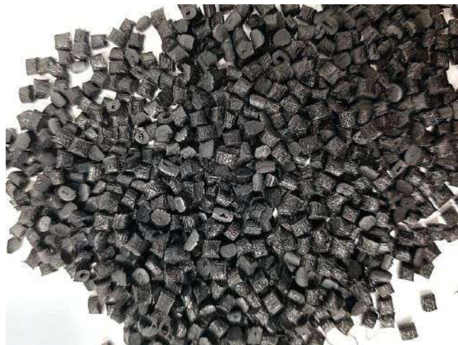
FIG 6 Are voids in the pellets of different sizes and randomly distributed (suggesting a problem with degassing in the extruder), or are they all the same size and always located in the center of the pellet (“shrink voids” usually associated with insufficient cooling downstream of the extruder)?
