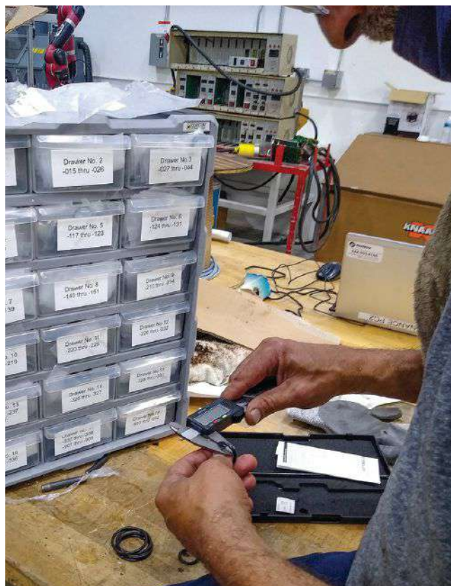
A service technician measures O-rings while servicing a hydraulic valve stack. (Photo: Garrett MacKenzie)
