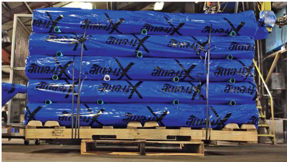
Tex-Trude is using Exceed XP 7 to produce 10-mil to 20-mil monolayer vapor-barrier construction films designed specifically for use under concrete slabs.
