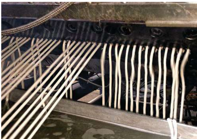
FIG 5 Spatial patterns are associated with product-quality defects as well as processing variables. Why does the product flow differently throughout the die plate? Why is the product hotter in the center of the die?
